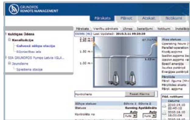
Screenshot of the GRM (Grundfos Remote Management) system, which offers a full overview of pump operation, performance and trends.
